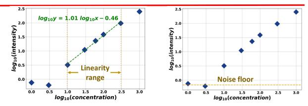
• The saturation point (if present) can be estimated as the concentration above which there is no longer an appreciable increase in fluorescence intensity.
