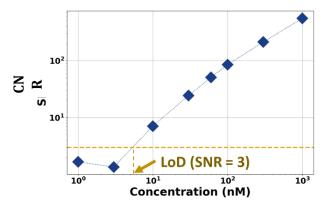
• Convert the background-subtracted intensities and concentrations to log scale in order to fit an equation of the form:
